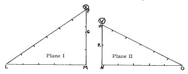
Two spheres, X and Y, of equal masses and radii, are placed on two inclined planes, as shown in the diagram. Neglect friction and air resistance, and assume that potential energy is measured from the level of points L, M, N, and O.
