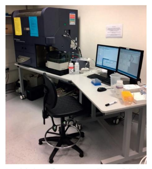
Figure 8.1 The photo shows a typical flow cytometry instrumentation with the cytometer itself and attached computer used for data acquisition. Underneath the flow cytometer are the sheath fluid tank and the waste tank.
